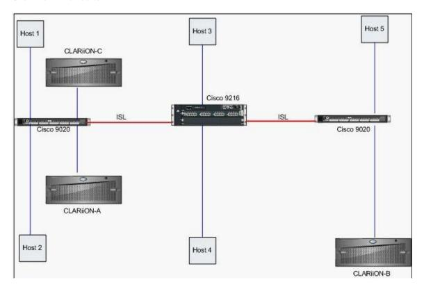
A customer is complaining that SAN Copy sessions from CLARiiON-A to CLARiiON-B take substantially longer than from those to CLARiiON-C. All hosts have 4 Gb/s HBAs. All Cisco equipment is base hardware configurations.
